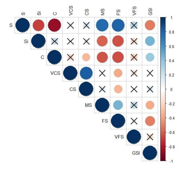
**Fig. 6.** Correlation matrix among Al<sub>2</sub>O<sub>3</sub>/SiO<sub>2</sub> ratio and particle size (S: sand; Si: silt; C: clay; VCS: very coarse sand; CS: coarse sand; MS: medium sand; FS: fine sand; VFS: very fine sand; GSI: grain size index (Al2O3/SiO2 ratio); level of significance is 0.05 and for insignificant correlations, coefficient crosses were added).
