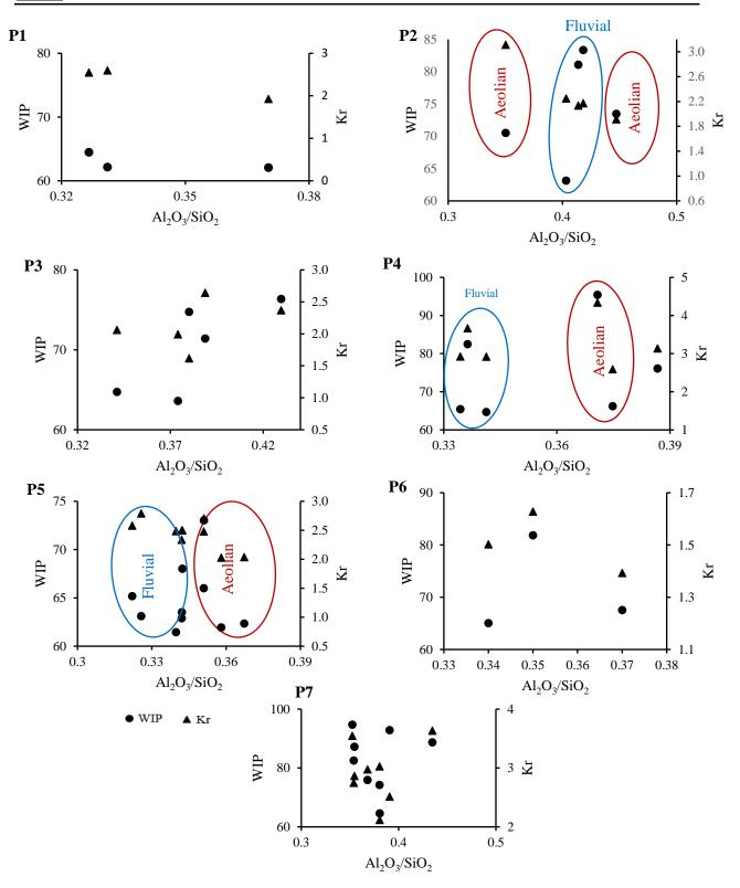
Figure 8. Relationship between weathering indices and Al<sub>2</sub>O<sub>3</sub>/SiO<sub>2</sub> ratio for the studied pedons
