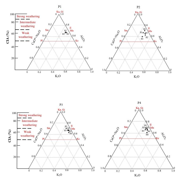
**Figure 7.** The Al<sub>2</sub>O<sub>3</sub>-(CaO + Na<sub>2</sub>O)-K<sub>2</sub>O (A-CN-K) ternary diagram for the studied pedons and their horizons. The position of minerals plagioclase (Pl), K-feldspar (Ks), smectite (Sm), illite (il), muscovite (Mu), Ka (kaolin), gibbsite (Gi) is given in the orientation of the ternary diagram. Hi (i=1, 2, ..., n) shows the number of horizons in each pedon
