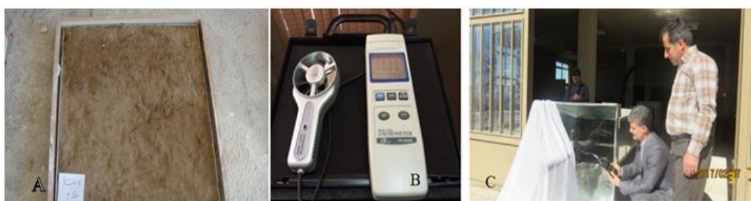
Fig. 2. A: Soil sample, B: Anemometer, C: Wind tunnel
