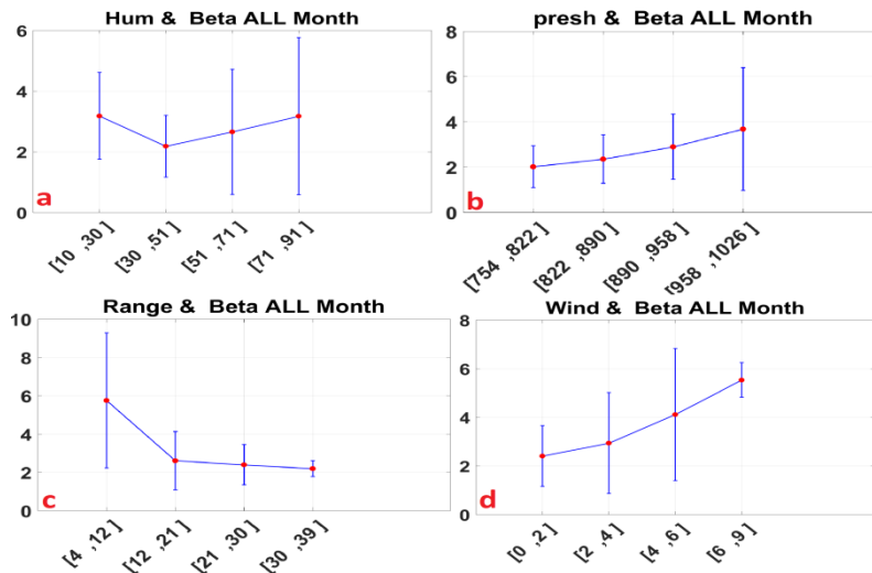
Fig. 12. The variation bars of mean and standard deviation of relative mean diurnal air temperature against different \beta classes in one year; a) humidity, b) pressure) mean diurnal temperature range, d) wind
