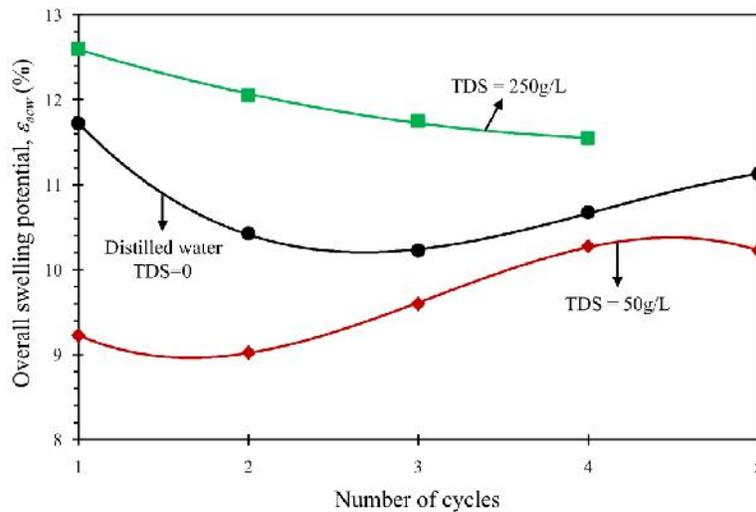
Fig. 6. Variations of overall swelling potential of soil samples during various cycles of wetting
