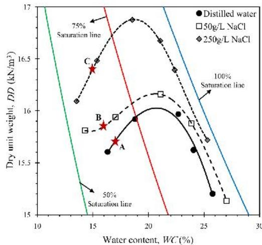
Fig. 2. Standard compaction curves for distilled water, 50 and 250 g/L NaCl solutions
