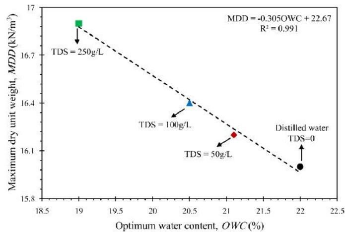
Fig. 4. Variations of maximum dry unit weight with optimum water content for various salt (NaCl) concentrations
