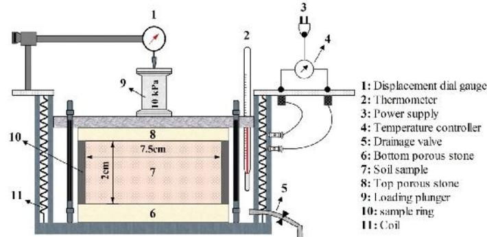
Fig. 1. Schematic layout of the modified oedometer apparatus
