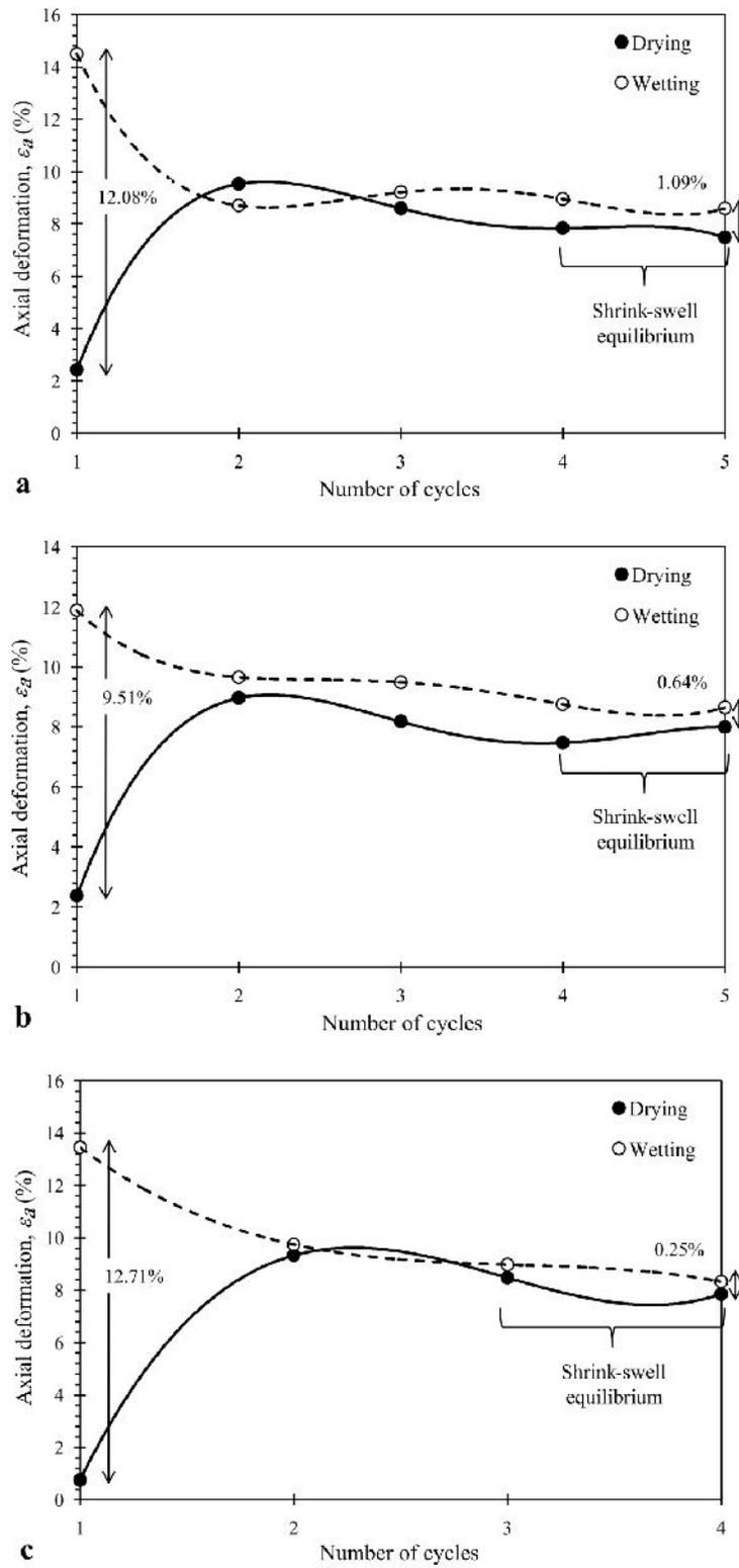
Fig. 5. Variations of axial deformation (shrinkage and swelling) of soil samples during different cycles of drying and wetting for (a) distilled water (b) 50g/L NaCl solution and (c) 250g/L NaCl solution
