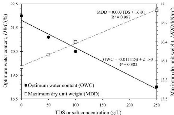
Fig. 3. Variations of optimum water content and maximum dry unit weight with various salt (NaCl) concentrations
