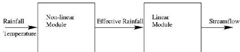
Fig. 4. Generic structure of the IHACRES model, showing the conversion of climate time series data to effective rainfall using the non-linear module, and the linear module converting effective rainfall to stream flow time series
