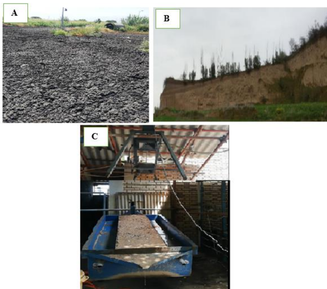
Fig. 2. The pictures of sewage sludge (A), The loess soils of Saadabad (B), and pressurized rain simulator (C).
