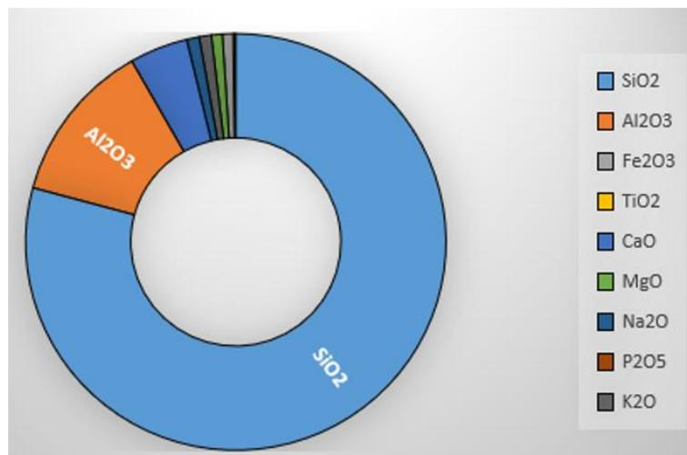
**Fig. 3.** The components of Zeolite.
