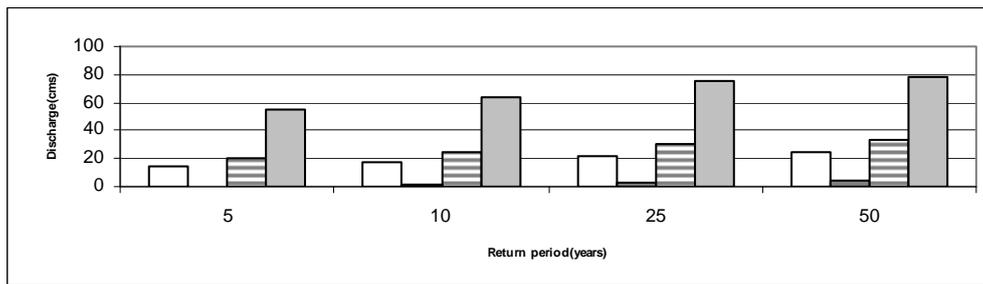
Fig. 3. Comparison of peak discharge obtained from innovative method and datum debit in sub basin of Barikan T3 (m<sup>3</sup> / s)
