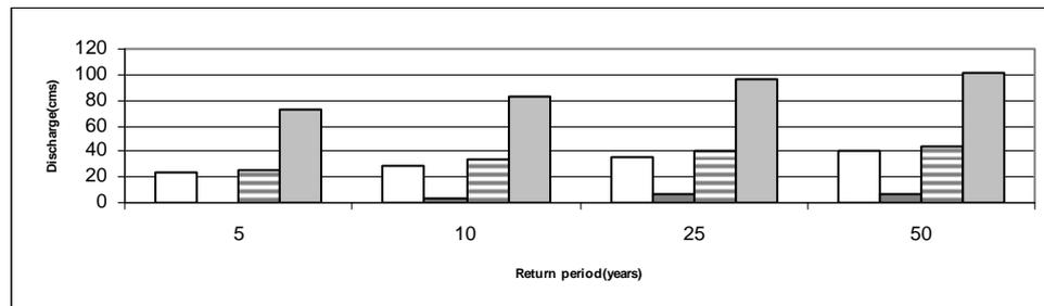
Fig. 2. Comparison of peak discharge obtained from innovative method and datum debit in sub basin of Varkesh T2 ( $m^3 / s$ )
