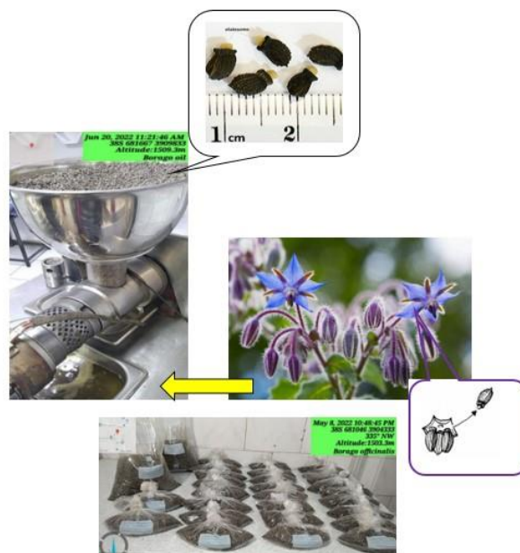
Fig. 2. Cleaning Borago officinalis L. seed after harvesting and extracting seed oil by cold press method
