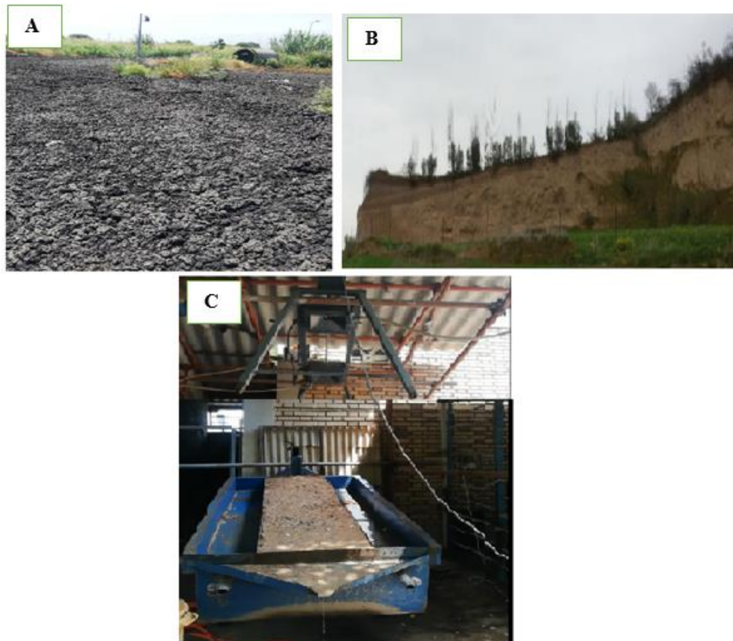
Fig. 2. The pictures of sewage sludge (A), The loess soils of Saadabad (B), and pressurized rain simulator (C).
